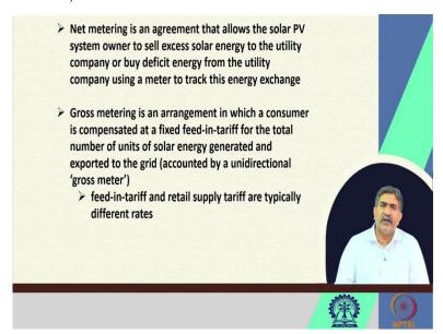
Now, net metering, gross metering, what it is and how it operates and whether it is beneficial for the renewables or not is something let us look at; net metering is about allowing the producer of renewable to supply the electricity to the licensee and accordingly, get the adjustment in the billing.
