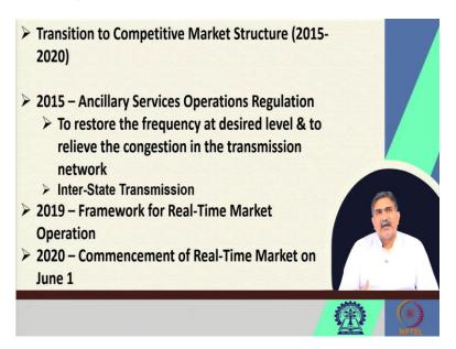
Now, you would find that certain developments have taken place also between 2015 to 2020. One important development is ancillary services operations regulation. This is all about bringing in a sort of mechanism where the congestion in the transmission network is to be addressed. So that, any situation of destabilizing the grid would be addressed by either generating units or by the licensees.
