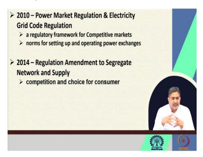
Now 2010, you again find that electricity grid code regulation has come into effect, and this is for making the power exchange market more robust; the idea is that. We know very well that now, grid frequency has been stabilized between 49.5 to 50.05, and this is what is the frequency in which the grid has to be maintained.
