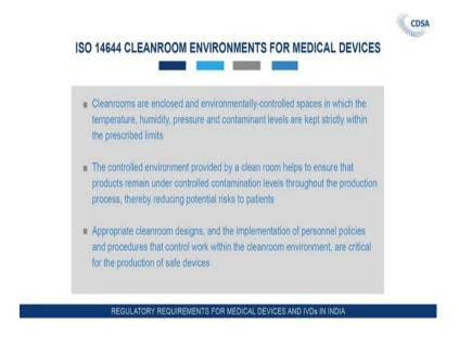
Cleanrooms are enclosed and environmentally controlled spaces in which temperature, humidity, pressure and contaminant levels are kept within strict limits. The controlled environment provided by a clean room helps to ensure that products remain under controlled contamination levels throughout the production process thereby reducing potential risks to patients.
