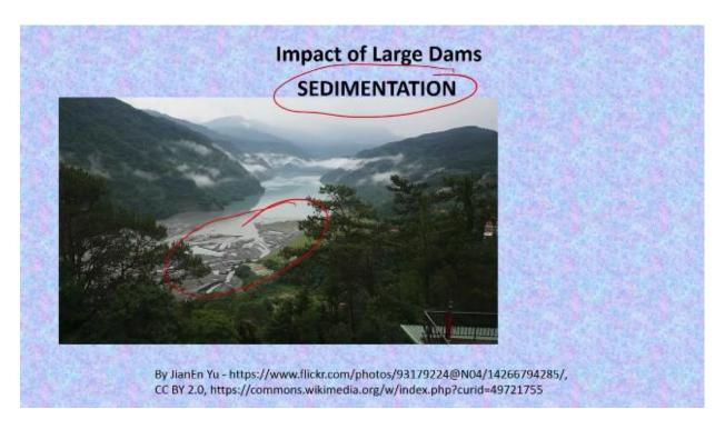
Now this sediment deposition in the reservoirs is something that we need to worry about because as the sediment gets deposited it starts reducing the storage available in the reservoir and that way it may reduce the life of the reservoir, the useful life of the reservoir itself, for example, this is the Gibraltar dam in the US.
