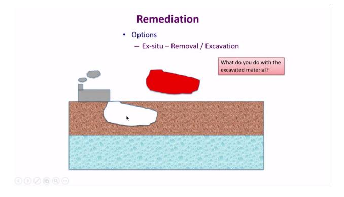
So, there is a possibility that exists we can do what is called as an Ex-situ option. We can remove the option that we have is that of removal of this entire contaminated zone. So, we take it out by excavation and then there will be a gap here that will be filled up with any clean material or a filler or anything that we want to do, and it is possible to do this. I have shown it schematically here.
