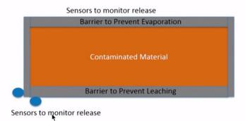
Monitored secure landfills are also used to store hazardous waste from industry and segregated hazardous components in domestic waste
