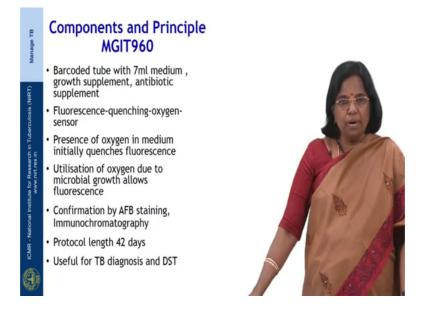
So, MGIT960 makes use of barcoded tube with 7 ml medium to which growth supplement and antibiotic supplements are added. Every tube has a fluorescence quenching oxygen sensor at the bottom, in presence of oxygen in the medium initially quenches fluorescence and utilization of oxygen due to microbial growth allows the fluorescence to be detected.
