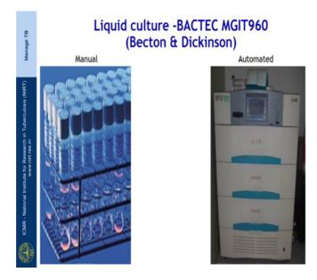
Next we come to the liquid culture based commercial system; the most widely used system which is the BACTEC MGIT960 from Becton and Dickinson. Two versions are available one is the manual version and the automated version which is the actually the MGIT960 system.
