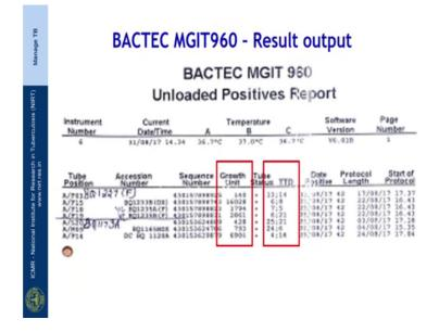
Now, this is an example of the result output from MGIT960; while it gives a lot of information the most important to look for are the growth units which is an a measure of the fluorescence that is detected in each tube and it does not reflect the biomass that is available in the culture.
