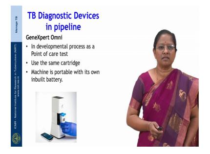
So, the next device that is in the pipeline is called as the GeneXpert Omni. So, this is still the developmental process as a point of care test, and it uses the same cartridge. The advantages that, it does not require a specialized laboratory facility for usage of this device, it is a portable device and it has its own inbuilt battery, but will be able to perform only one test at a time and the time duration is a same as that of a gene expert.
