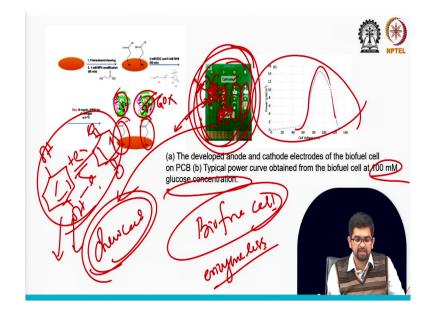
See here the design this is a PCB based cell power device PCB. So, here you can see the cathode and anode. So, anode here actually what we did see first we use some linker based on this linker we immobilize the glucose oxidase they are the glucose oxidase enzyme. So, in the
