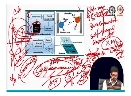
I am showing this one suppose this is your sensor surface you have some specific you are thinking your nanomaterial is very specific. So, here you are applying 0.3 volt for the chronoamperometric case, but in that potential if it is showing the glucose oxidations in your real sample content let us apply like different potential.
