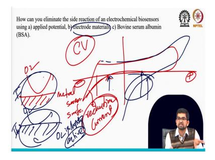
If you measure so, what you will do? You can measure a cyclic voltammogram on your sensor surface. Suppose you have a metal base metal base sensor right, surface. And you wanted to check the oxygen side effect oxygen, how oxygen is reacting on this sensor. What you will do? On the sensor in a buffer sample let us measure a cyclic voltammogram.
