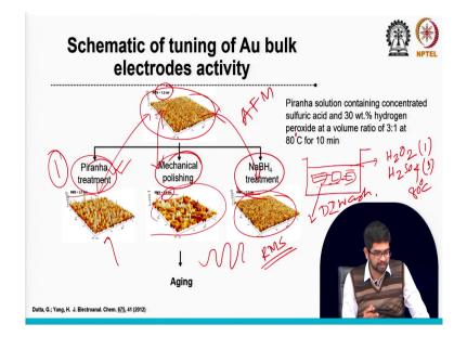
See here the schematic. So, I wanted to show you a basic concept of the different treatment, especially I am saying here the pre-treatment. One is the piranha, another is mechanical polishing and last one is sodium borohydride treatment, ok. So, let us show you. Piranha treatment, it is the solution that contain sulphuric acid and 30 weight percents of the hydrogen peroxide and this mixture is the 3 is to 1 ratio.
