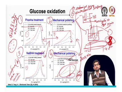
So, first you follow number 1 mechanical polishing. So, it is done. So, after mechanical polishing as you can remember and you have to keep your electrodes in the DI water then you have to sonicate it for 15 minute, then you can wash again the surface.
