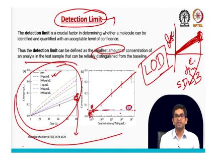
But, if suppose you have one biosensor and it can measure means you can it can measure 10 picogram per ml, here you can see I mean here you can see difference here 10 picogram ml here it is showing the difference. But, after calculating standard deviation multiplying with 3 everything, but your 3 times standard deviation line here and your 10 picogram per ml this charge is point is showing here then this is not your limit of detection.
