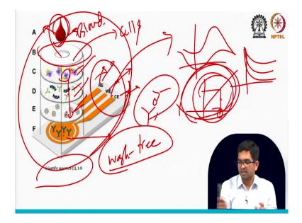
So, I will show you this kind of wash-free sensor can be useful very cheap base or lab on a cheap based biosensor like something like this I want to show you one basic very very basic example that is reported in this general. You can see here or your primary antibody coated your three electrode system, right? Reference electrode, working electrode, counter electrode – this is your three electrode system.
