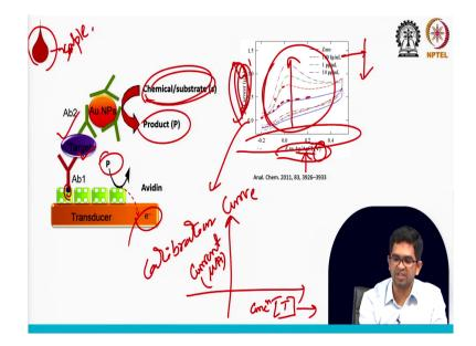
Now, I will come how we can measure this electron. See, in the cyclic voltammogram case, we will scan in a potential window like 0.2 to 0.4 and we will measure the different different potential we will measure the current. See when you oxidize from the negative potential to positive potential, the current increase and then it is become like this.
