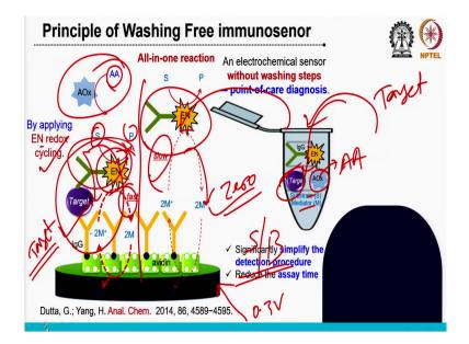
So, washing free technique this is the very important where all environments all the reactions will happen on the sensor surface you do not need any extra steps. Suppose you have a like this a sensor surface that already modified with some primary antibody that where I use the avidin and biotin avidin antibody this conjugation protocol.
