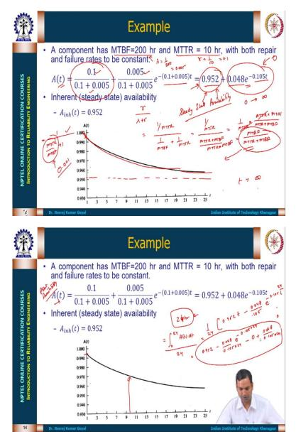
If I let us say if I plot it here. I have plotted it here. Let us say for an example, if I take MTBF is 200 hour and MTTR is 10 hour. So, that means lambda is equal to 1 upon 200 and r is equal to 1 by 10. So, that is equal to 0.005 and this is equal to 0.1. So, I will apply this formula r upon lambda plus r that is 0.1 divided by 0.1 plus 0.005 plus 0.005 divided by 0.1 plus 0.005 into exponential of 0.1 plus 0.005. So, this will become 0.952 plus 0.048 e to the power minus 0.105 into t.
