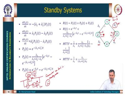
Now, if we look at standby systems. Standby systems means as we discussed earlier like of generator can be one standby system. In case of generative, what is happening we generally have the power supply so, power supply or electrical input is generally working. Now, so, we have the electrical supply coming from a state electricity board.
