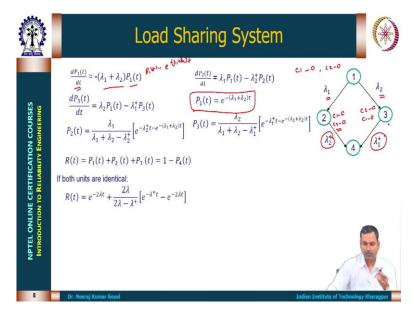
So, we have component 1 and component 2 like we discussed earlier, we have component 1 and component 2 both are operating here in state number 1. In state number 2 or state number 3, there are two possibilities here either component 1 can fail. So, if component 1 fails component 2 continuously operate here that is our system state 2. There is another possibility in place of component 1, component 2 fails. So, component 2 is failure, but component 1 is operating in this state.
