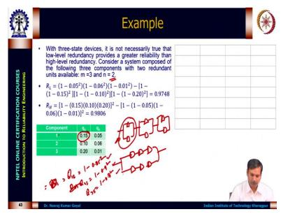
If we take an example here that if we have three elements here, 1 2 3 and N is equal to 2, that means, we have low level configuration and high level configuration. So, we have 2-2 elements here for low configuration and for high level configuration we have two parallel rows, 1 2 3, 1 2 3 and I want to calculate the reliability for this. Now, for this, we know that
