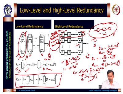
Similar concept is applicable when we discuss with the low level redundancy and high level redundancy. For low level redundancy means, see, if the system requires M element like M can be let us say if M is 4 where we were discussed earlier that we need let us say antenna, we need a transceiver, we may need a power supply right. Let us say M equal to 3. So, what can happen? In low level redundancies, let us say N N elements.
