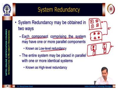
Generally, system may be having a different way of redundancies, like you have multiple components with available video. So, for to get the system function you can connect them as in parallel system.
