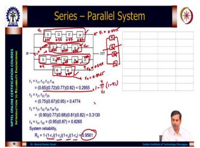
One is series parallel system. So, it is series combinations which are connected in parallel. If we see here, so here we have series of 4 components here, series of 3 here, series of 5 here, series of 2 components here, these components are connected in parallel. Now we want to know the reliability for this. So, to solve this, first generally we solve the series components.
