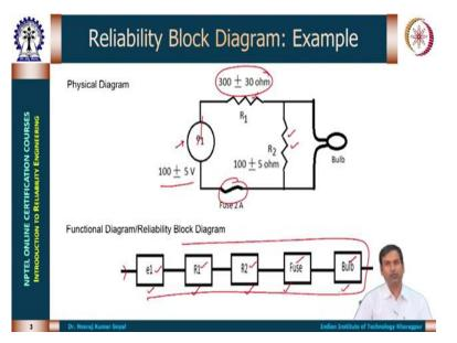
Let us say we want to understand what is the reliability block diagram let us see if we have a simple voltage divider circuit like this where we have a supply voltage we have two resistances, one is this resistance another is this, R1 is here R2 is here and we also have a fuse we have the bulb connected across the R2. So, whatever voltage is here this will divide and whatever voltage comes as output that will be used for the bulb.
