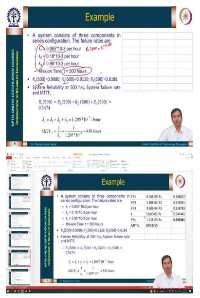
$$R_{s}(500) = R_{1}(500) * R_{2}(500) * R_{3}(500) = 0.5474$$
