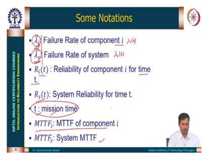
Let us see some notations which we will be using throughout, we will try to stick to this lambda i lambda i is the failure rate of component i. So, each component i will be having a failure rate. So, whenever we are using exponential distribution, we know it is having the constant failure rate. So, each component failure rate we will be representing by lambda i. So, if I say i equal to 1 this will become lambda 1 equal to 2 it will become lambda 2 like that.
