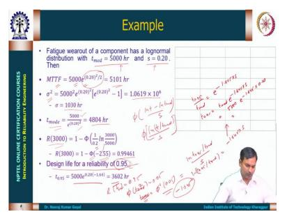
Now, let us take an example here to understand that how we can calculate this? So, for calculation purpose, let us see, we have taken an example, that fatigue wearout of a component follows the lognormal distribution and the parameters given a t median that is equal to 5000 hours and S is equal to 0.20. So, if we have these 2 parameters, we know full about the lognormal distribution now. So, we can calculate everything what is MTTF?
