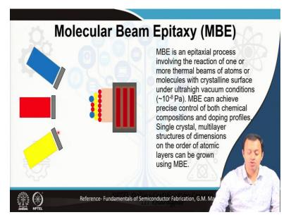
So, how do we obtain one such way in which this ultrapure atomic scale pure wafers substrates can be done is using this technique called molecular beam epitaxy. Molecular beam epitaxy involves thermal beams of atoms, molecules beams of atoms that are put through a chamber that is under an ultra-high vacuum condition 10 to the power minus 8 pascals.
