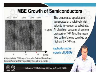
So, this is something at an atomic scale you can see these are the molecules of aluminum arsenide, these are the molecules of gallium arsenide. And look how nicely, these are molecule by molecule step by step arranged in a planner direction and this entire distance is nanometers. So, the overall within 10 to 15 nanometers, you have an alternating gallium arsenide and aluminum arsenide or aluminum gallium arsenide being formed.
