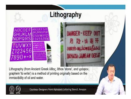
So, this is your stencil. I even got it these images from Amazon as such. This is the stencil. You spray paint over it. Selectively the paint passes through these holes, these stretches, and you get some amount of letter coming out. Rest of the place the paint is blocked and it remains as it is. So, this is what a stencil can do. You can utilize stencils to make printing, make some kind of a message, make some kind of an image, make some kind of a picture.
