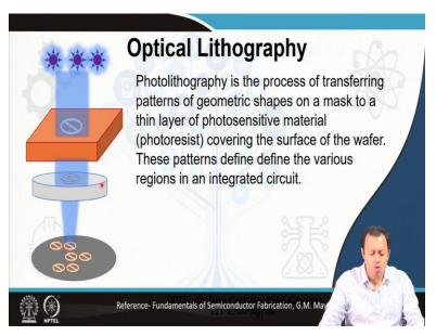
What is the procedure? Photolithography is the process of transferring patterns of geometric shapes on a mask, mask is the stencil here, to a thin layer of photosensitive material, a photoresist, that covers the surface of the water. These patterns define, I put define twice, the various regions in an integrated circuit. So, what is the overall procedure? I have a cool animation for you, which I made myself.
