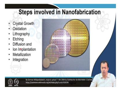
So, let us try to see what are the different processes involved in nanofabrication. These are the several different process of nanofabrication and they are but a typical example. We start with crystal growth, i.e. growth of a silicon chip. Then we oxidize, so that silicon becomes silicon dioxide. We have lithography which is patterning, etching.
