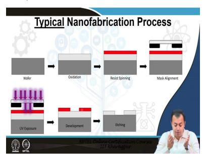
So, we start with some kind of a wafer. Wafer is basically a piece of silicon which has been polished. How do we make, it is a pure piece of silicon? Usually, silicon, but it could be glass. It could be gallium arsenide. It could be other exotic materials. It starts using with a wafer. Wafer is the starting piece, the, what we go for microfabrication. How this wafer is made?
