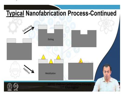
What next? Well, there are two processes. Either you go for subtractive, as I said. You eat away the silicon part and make a hole in the silicon. Remove the glass altogether. And now you have a patterned silicon. Or additive, where you put some sort of a metal in those trenches.
