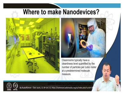
Where exactly are these nanodevices made? The nanodevices are made in specific rooms, specific laboratories, specific environmentally controlled areas, which we call as clean rooms. They typically have a cleanliness level quantified by the number of particles per cubic meter. So, the total number of dust particle per cubic meter of this air at any time gives you the class of this material and you wear these sophisticated suits. Nowadays, we call it PPE, personal protective equipment.
