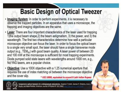
You need to have a specific power. Say, for example, 3 joules, 3 milliwatt giving you something like 4 to 5 joules per centimeter square. And if it is working at a wavelength of say, 1043 nanometer, you can easily trap cells, because these are the usual frequencies, near infrared frequencies where cells or biological matter for that regard, most biological matter for that regard do not absorbed. So, basically you need three things, an imaging system, a laser and an objective.
