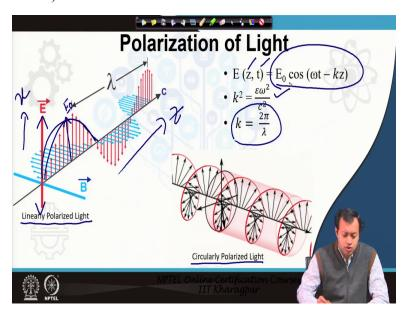
So, since we are mostly describing light from the point of view of it oscillating electric field, there comes the term polarization, polarization describes how the oscillating electric field behaves with respect to the propagation of the light. The two most important parts the two most important definition of polarization or the variety or the type of polarization that I want to discuss is linearly polarized light and circularly polarized light.
