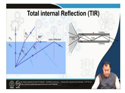
And how do they work? Well they work by this concept the light is guided through the core, that is the optically dense material, do not fall for the color, this is denser, this is rarer, this has a higher refractive index, this has a lower refractive index, the light is guided, I think I discussed it a little bit before by the process of total internal reflection, what does total internal reflection means, all of you know it from your high school but I will just revise you once again.
