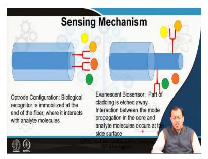
I will give you a bit more detail on the sensing mechanism part, what is the sensing mechanism, you have first the Optrode Configuration. The one which I showed single point, where the output you have put these kinds of antibodies, these kinds of immobilizer, these kinds of biorecognition units which are specific to a specific pathogen or an analyte only and when these gets attached there is a change in the overall refractive index.
