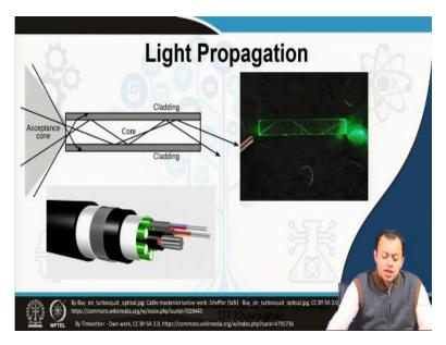
So, this is how, this is a depiction like that, this is an acrylic fiber and you have sent a laser light and you see it simply bounces of its surface and go through without any of the light going to the surface or very minimum amount of light going to the surface, this is a typical real-life example. So, if this laser light contains some sort of an information at the input that information could be decoded or received at the output.
