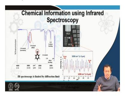
However, when it comes to getting chemical information, we mostly rely on spectroscopy i: e molecular vibration and you know molecular vibration happens at infrared. So, if your molecule or if your nanostructure is of a size of say less than infrared, you start getting diffracted limit. Yes, I told you that there is evanescence field by which you can measure, but evanescence field as I said by definition is weak and when you try to artificially amplify it you get into several different trouble.
