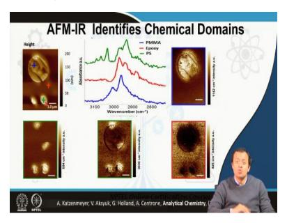
Same example, start from the beginning, you have epoxy, bigger sphere PMMA, smaller sphere polystyrene, we purposefully made it, naturally occurring will have random distribution, this is also randomly distributed but just by looking at under a microscope we can identify bigger sphere as PMMA, smaller sphere as polystyrene, in an epoxy matrix, three different chemical species and all three chemical species absorbs different light.
