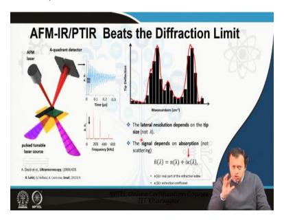
What do we do? We used the AFM-IR or PTIR technique, this is something that I myself personally did, I do here at IIT Kharagpur, what I do I put my sample on top of a prism, the prism is transparent, I put my sample on top of a prism and this sample is scanned in x and y direction, this direction and this direction by this AFM laser.
