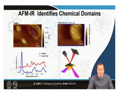
So, we started with a known sample, everything when you are trying to establish, the proof of concept you start with a known sample. We start with a sample that has three different chemical domains, you have polystyrene, small spheres, PMMA polymethyl methacrylate, large spheres and epoxy resins these are three different chemical species, epoxy resin the red one, polystyrene and PMMA and you get a height image of it,
