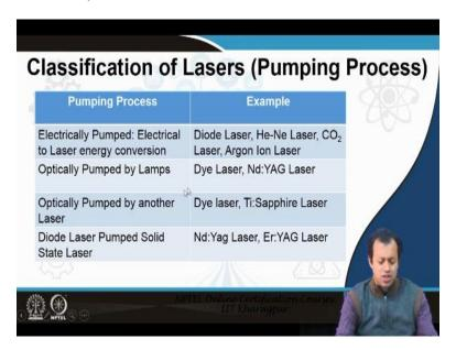
So, let us classify the lasers, the lasers can be classified according to their pumping processes, electrically pumped, electrical to energy laser energy convention, diode lasers are usually electrically use voltage to for the electrons to go from lower level to higher level, helium neon laser, CO2 lasers, remember CO2 is not electronic, it is molecular, you have optically pumped by lamps, you shine light on it and thereby electron moves up.
