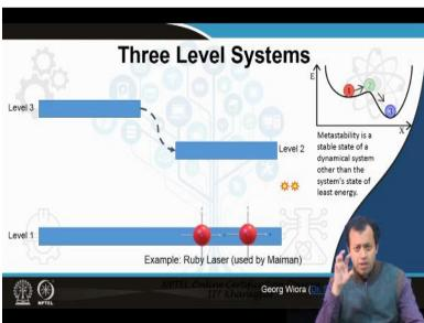
Let us have a three level system, a third level is added, though I am calling it level 2 because these numbers determines the energy, you have level 1 with the lowest energy state, level 3 as the highest energy state and level 2 as the intermediate energy state which is a metastable state.
