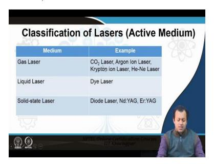
Similarly, medium, what is the active medium? It can be solid, liquid, gas, you have CO2, Krypton, Argon laser, Helium Neon laser these are gaseous laser, where the active material is actually gas, why not gas, why cannot as long as it has atoms, as long as it has energy levels gases have as a good energy levels, you have a container 2 mirror container, 2 at the end like a tube, you have put 2 mirrors in between them and it has gas in between, so why not, why cannot gas laser work.
