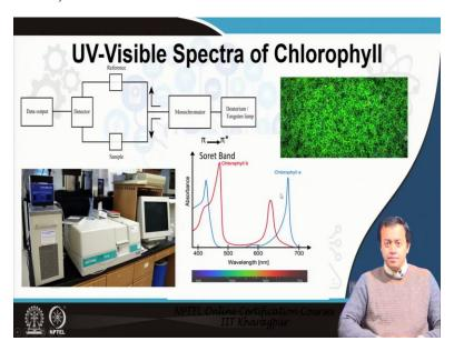
A common example of such UV visual visible spectroscopy is detection of chlorophyll. Several of you might have seen this UV visible spectrometer present somewhere in your lab. How does that work? It has a source, a tungsten lamp, it passes through a monochromator. What does monochromator do? Monochromator provides, it filters basically a light filter, mono means one chromator means color.
