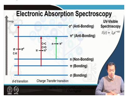
Electronic absorption spectroscopy is also called UV visible spectroscopy or as you cool kid will say UV vis spectroscopy. I think several of you already have seen a UV vis spectrometer. UV vis spectrometer is quite common to have in colleges and universities and labs. So, UV vis spectroscopy deals mostly with the transition of electron in a molecule moving from lower level to higher level, lower energy level, lower energy state to higher energy state.
