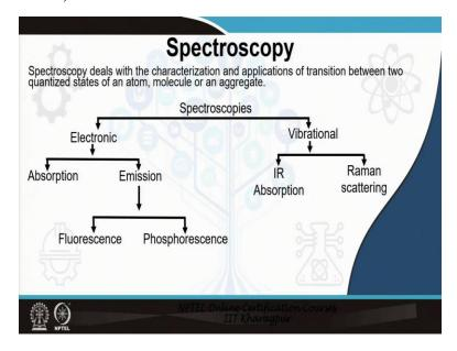
Spectroscopy is the branch of science which mostly deals with characterization and application of transition between two quantized states of an atom molecule or aggregate. Now, what does that actually mean? It simply means, that molecules or part of molecules absorb light. Molecules or part of molecules, what do I mean by part of molecules I means electrons, electrons are parts of atoms electrons are parts of molecules.
