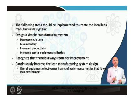
The following step should be implemented to create the ideal lean manufacturing system. Design a simple manufacturing system it should be simplified. Decrease cycle time, less inventory, increase productivity, increase capital equipment utilization. Meaning if you have machines try to see that it is always under utilization, not under utilize always being utilized.
