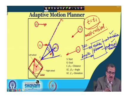
Now, to start with let me take a very simple example of one mobile robot. And this particular mobile robot is nothing, but actually a two wheeled robot. So, this is actually your the robot that two wheeled robot. So, here I have got one wheel, I have got the second wheel here and for support actually I have got a caster here. So, caster is actually one wheel, but it has got no drive unit and supposing that to operate. So, these two wheels say I am using say two DC motors.
