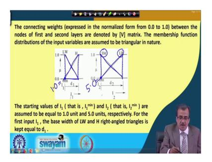
The connecting weights are lying in the range of 0 to 1 and if you see the membership function distribution which we have considered for the two inputs like I 1 and I 2 are as follows. Now for simplicity we have considered like the low I 1 is nothing, but this. So, this type of membership function distribution right angle triangle and for the high another right angle triangle and there is overlapping also.
