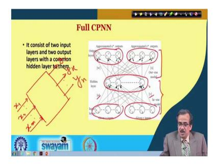
Now, this is actually the schematic view of the full CPNN and if you see construction-wise, it has got two input layers. So, I have got one input layer here. So, one input layer, here I have got another input layer here, then we have got two output layers so this is one output layer, another output layer and we have got actually a common hidden layer and this hidden layer is denoted by this. So, we have got two input layers, two output layers and one hidden layer.
