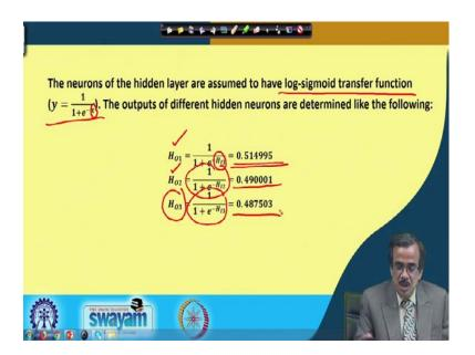
Here, we have got this particular transfer function, that is your the log sigmoid transfer function and that is nothing, but  $y = \frac{1}{1 + e^{-x}}$ . So, this particular x is actually I will have to put the input of the different hidden neurons. Now, this  $H_{O1} = \frac{1}{1 + e^{-H_{I1}}}$  and if you put this numerical value and solve there is a possibility that I will be getting this particular the output.
