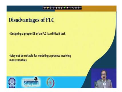
So, here to discuss the demerits actually, what I do is so, we try to say that the performance depends on the knowledge base and how to determine this particular optimal knowledge base; that means, how to determine the database, how to determine the optimal rule base? So, that is a difficult task, the fuzzy reasoning tool, in fact, does not know anything, it does not have any in built optimisation tool.
