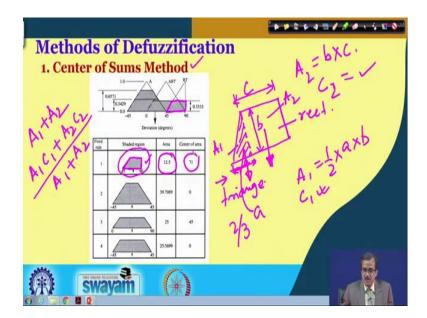
Now, the first method for which I have already discussed the principle, and now I am just going to apply to solve this numerical example. Now, the first method, this particular method is your the center of sums method, now let us see according to this, how to determine the crisp output. Now, if you see corresponding to the different fired rules, we will be getting the different shaded regions as the fuzzified output; for example, say if I concentrate on this particular output first.
