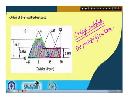
And, as I told, our aim is to determine what should be the crisp output. And, to determine the crisp output actually, we will have to take the help of defuzzification. Now, I am just going to discuss the different methods of defuzzification. Now, let us try to concentrate on the methods of the defuzzification.
