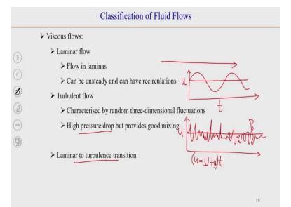
Now, so we have been talking about laminar and turbulent flows quite often and we will be talking about. So, the next classification we will look at is a laminar and turbulent flows. So as the name suggest laminar, so laminar means lamina, lamina means layers. So, laminar flow is when the flow or the fluid is flowing in laminas, so the flow is smoothly in parallel laminas and there is no transfer of momentum or there are no velocities or no eddies which causes mixing.
