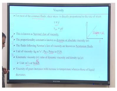
So, let us define viscosity. And viscosity is basically it is, it can be defined or it is defined for the fluids where there is a linear relationship between stress and rate of strain. And that is common for most of the fluids. So, we talk about the two most common fluids that we are concerned with which is water and air. Both of them they show this property that the shear stress is directly proportional to rate of a strain.
