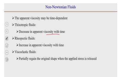
Now, time dependent fluids. So, all the Non-Newtonian fluids we talked about they show, time independent behavior that their viscosity does not change with time if the shear rate or the rate of strain is constant or if the shear stress being applied on them is constant than the viscosity does not change with time. But there may be or there are some class of fluids which shows time dependent behavior that their viscosity changes even when the shear stress or rate of strain is constant.
