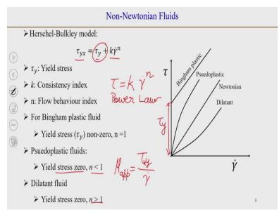
There are some fluids for whom which so the time dependent behavior but before that we can characterize this the flow of Non-Newtonian fluids in terms of mathematical models. So, a common general model we can write down where, the stress is equal to yield stress plus k strain rate raise to the power n. So, it shows the yield stress behavior and nonlinear relationship or power law relationship between stress and rate of strain.
