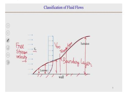
So, we will be using this term boundary layer quite often this course. So, what is boundary layer? The most common example or the easiest way to understand boundary layer is considering flow over a flat plate. So, we have a flat plate here which is a solid wall. And the flow approaches in a over this flat plate. The flow, let us say you have a the flow of air on land. So, this air approaches with a velocity  $V_{\infty}$  which is often termed as free stream velocity.
