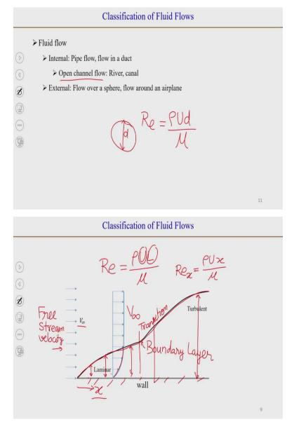
The next classification we will just look at what is called internal flow. So, internal flow is basically flow in closed conduits, close channels, close pipes and that is what we will look at in this course quite often. There is another class which we can call open channel flow. So, when we talk about
