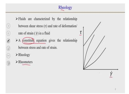
There is this name Rheology which is basically the study of relationship between stress and rate of strain. When we defined a fluid we said, a fluid is defined as a material which undergoes deformation continuously when it is under a shear stress. So, when we apply a shear stress on a fluid it deforms continuously.
