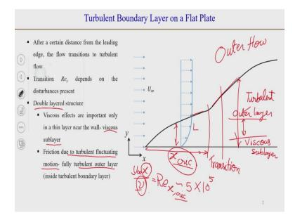
So, this is typical image for a boundary layer over a flat plate that we have been discussing. So, this is the laminar boundary layer and here you have a turbulent boundary layer. Of course, you can see that the turbulent boundary layer is significantly thicker than what you have, say for laminar boundary layer. So, turbulent boundary layer is thicker. The slope you can see here, the slope is smaller and slope in the turbulent flow is significantly larger.
