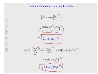
Now, we can rearrange it in a simpler form. So, we can do this and we will get  $\delta = \text{Re x}^{-1/7} \times \text{x}$  multiplied by some constant. So, that will give us  $\delta/x = 0.16 \text{ Re x}^{-1/7}$ . So, we get a relationship for turbulent boundary layer thickness.
