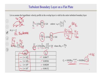
This is the logarithmic velocity profile, which is basically u bar/u  $\tau$ , which we call u + also, is equal 2.5 times ln, y u  $\tau/v$  + 5. So, this is also called y + yu  $\tau$  y v. When y =  $\delta$ , so that means, where  $\delta$  is the disturbance thickness or boundary layer thickness, so at this region, at this point, if the free
