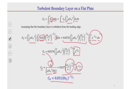
Now, we know the skin friction coefficient, we know the boundary layer thickness, we could also calculate what is the drag on a flat plate. Let us say, where the turbulent boundary layers starts from x = 0 itself. So, that will be  $\tau w \times b dx$ , where b is the plate width normal to the screen. So, we can write  $\tau$  w in terms of Cf  $\times 1/2 \rho U_{\infty}^2 \times b dx$  and then we can replace the value of Cf there.
