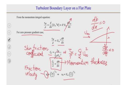
So, let us look at the turbulent boundary layer on a flat plate. And we will consider that this plate is smooth, there is no pressure gradient along the flow direction. So first, we will write down the momentum integral equation. So, this momentum integral equation, we derived when we looked at the boundary layers. So, in this, if we say that the pressure gradient is 0, so from because in the boundary layers, when the pressure gradient is 0. So, that means, dp/dx = 0.
