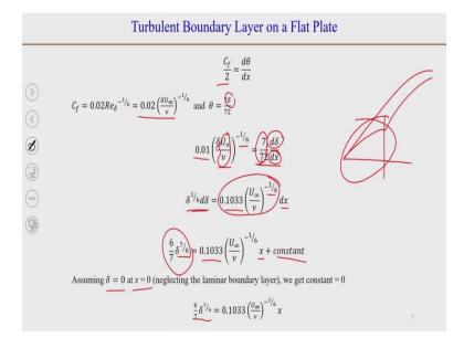
So, now we have Cf in terms of  $\delta$ , we have  $\theta$  in terms of  $\delta$ . We can substitute both. So, when we substitute in this then this del, Cf/2 will become simply 0.01, Re  $\delta^{-1/6}$  or we can write Re  $\delta$  in the expanded form, where we have  $\delta$  explicitly, U<sub> $\infty$ </sub> and v are constant. This = 7/72 d  $\theta$ /dx. So, this will be d  $\delta$ /dx.
