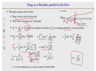
If you have a flat plate parallel to the flow, in this case because the plate is very thin So, the frontal area actually negligible and in this case the drag because of the pressure will be negligible because the pressure forces along the x direction will be 0.
