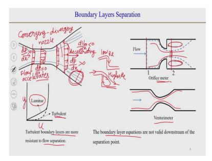
So, there are a number of such cases. One case is for example you have a converging diverging nozzle and you have an incompressible flow. So, in this region where the flow is accelerating because the area available for the flow decreases, So, the velocity will increase and the flow will
