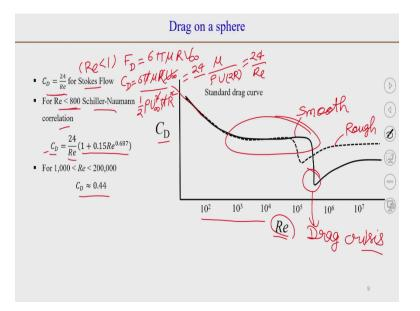
And we can also see that how the drag on a smooth sphere varies with Reynolds number. So, this is drag on a smooth sphere and then a qualitative representation for a sphere, which is rough, but it will depend also on the roughness of the sphere. So, you can see that at very low Reynolds number it will follow the Stokes law which is CD = 24/Re.
