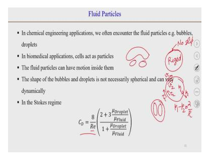
So, when you have fluid particles for example bubbles or droplets or when we talk about biochemical applications they might be cells. So, in these cases, when we talk about a rigid sphere, the boundary condition at the surface of a rigid sphere is no slip, whereas, if it is rigid, but if you have a fluid sphere then you have a continuity of velocity and the continuity of shear stress and the normal stress. So, p1 - p2 =say if it is spherical 2  $\sigma/R$ .
