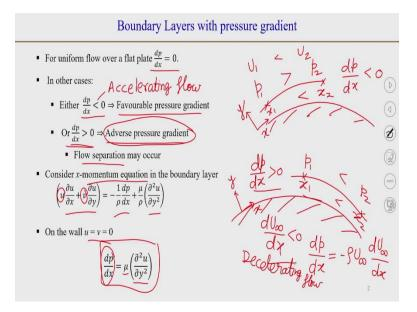
So, we said that when the flow is uniform over a flat plate dp/dx is equals to 0, but if this is not the case then it might be either less than 0 or greater than 0. So, if you have a boundary and on that boundary if the pressure is changing from p1 to p2 and the x direction is along the boundary and y direction is normal to it. So, these points let us say x1 and x2.
