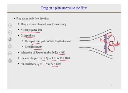
Now, we can consider the other case where the plate is placed normal to the flow. So, in this case there will be viscous drag or there will be viscous force on the plate, but that will not be along the flow direction, So, that will not be called drag. So, when we talk about drag that will be only because of the pressure difference say p1 on this side and p2 on this side.
