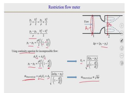
Now what we need to find is is the flow rate, so we can relate it that the pressure difference is already known to us. So, we can rearrange this equation in terms of pressure difference, p1 - p2, which is what we will measure  $\Delta p$ , p1 - p2. We will put a pressure tap here, a pressure tap here and connect it with a manometer. So, we will be able to measure the pressure difference.
