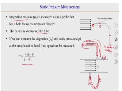
In this case, you can use the manometer again. It should be aligned so that the flow which is coming here it can be stopped and you can measure the stagnation pressure. And this device is known as Pitot tube. So, what we have seen is that you can measure stagnation pressure using the Pitot tube.
