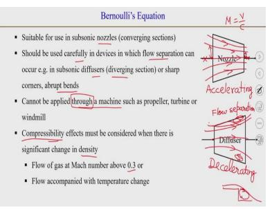
Now one of the common applications we can do it is in nozzles, so nozzles can be when the flow is subsonic. So subsonic means that the Mach number of the flow. If you remember the Mach number is basically M = V/C, where c is speed of the sound. So, if the velocity of the flow is less than velocity of the sound in that medium under the flow conditions at the same pressure and temperature then the flow is subsonic when Mach number is less than 1.
