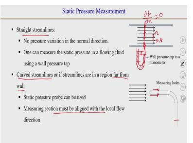
Now as I said that we will discuss some measurements also here. So, one can measure static pressure by simply in a flow where the streamlines are straight. So, as we discussed, when we discussed Euler's equation that if the streamlines are straight then  $\partial p/\partial y$  or  $\partial p/\partial n$ , when we talked about the in the streamline coordinates that was a function of radius of curvature.
