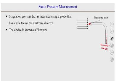
Now you can measure stagnation pressure. So, to measure stagnation pressure, you can put a probe in the flow and if you measure the pressure at the point at the front, so which will act as a stagnation point because this the flow may enter from here, but remember that this is connected to a manometer or to the hands of a manometer.
