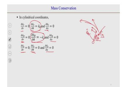
Now so if we write down the derivatives of all the variables, all the unit vectors in the cylindrical coordinates, so the unit vector, the differentiation of  $e_r$  with respect to r  $\theta$  and z is 0. The derivatives or the partial derivative of  $e_{\theta}$  with respect to r and z, they are 0. The partial derivative of  $e_z$  is 0 with respect to all the variables, r  $\theta$  and z. There are only 2 partial derivatives which are nonzero here and we can understand that.
