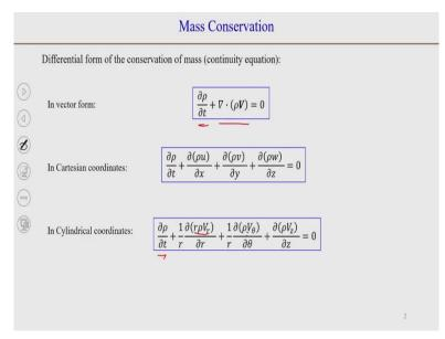
So we will look at the conservation equation in the cylindrical coordinate system here. So, if we write down the mass conservation equation in the vector form,  $\frac{\partial \rho}{\partial t} + \nabla .(\rho V) = 0$ , which is
