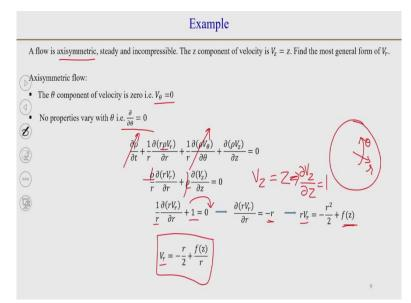
So, now we will look at a simple example, which asks us that if flow is axisymmetric, it is steady and incompressible. The z component of velocity has been given which is  $V_z = z$  and we have to find the form of  $V_r$  or the radial component of velocity. So, we already know what is a steady flow? That means  $\frac{\partial}{\partial t}$  is 0, so the unsteady term is 0, when the flow is incompressible, density is constant.
