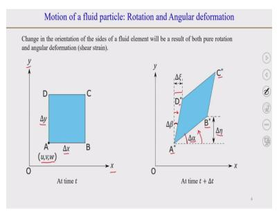
So, let us consider a fluid element which is rectangular, even though it appears to be square, we will assume it to be rectangular the side AB is of length  $\Delta x$  and side AD is of length  $\Delta y$ , the velocity components in the x, y and z direction at point A are u, v and w and this is a 2 dimensional fluid element in xy plane. It is named as, the corners of the fluid element are named as A, B, C and D, this is at time t.
