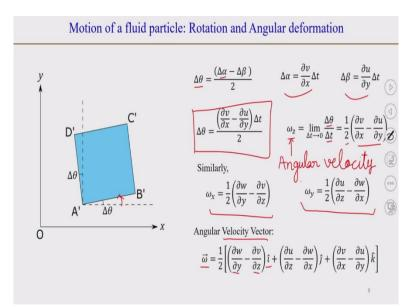
So, we can substitute those values. So, first we substitute or first we find  $\Delta\theta$ , where  $\Delta\theta$  is the rotation of the fluid element. So,  $\Delta\theta = (\Delta \alpha - \Delta \beta) / 2$  and we can substitute these two values of  $\Delta \alpha$  and  $\Delta\beta$  in here. So, we get when we substitute for  $\Delta \alpha \partial v / \partial x$  into  $\Delta t - \Delta\beta = \partial u / \partial y$  into  $\Delta t$ .
