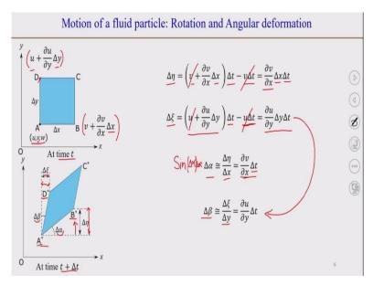
Now, as we said earlier that let us assume that the velocity of the fluid at point A is u, v, w and what we need to see is that what is the movement or what is the displacement of the fluid element or what is the displacement of point B from its previous position or with respect to point A. Similarly, we also need to see what is the movement of point D with respect to point A.
