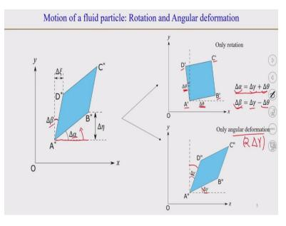
So, let us see if we assume that the pure rotation of fluid element or rotational component it has rotated let us say by an angle  $\Delta\theta$  and if there would have been only rotation then these the points of the particle would have been on the location A', B', C' and D'. Now, if it had been only angular deformation, then the angle would have changed by a magnitude of 2  $\gamma$   $\Delta$ .
