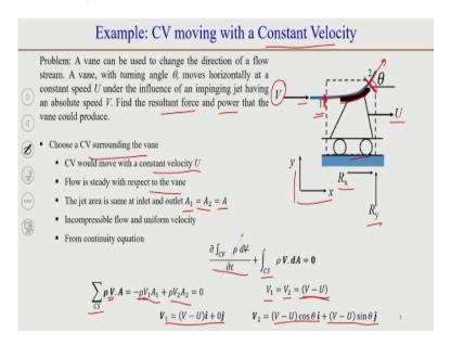
So, let us look at the next problem. Now, in this problem we will consider a case where the control volume moves with a constant velocity. So, if we have a vane, vane is generally a device which can turn the flow, so this is the vane and a jet hits this vane and the flow is the direction of flow is turned from up, so it comes along x direction but then it turns at an angle  $\theta$  from the horizontal edge, we can see from this figure and this vane is connected with the trolley.
