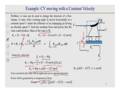
Now, we have been able to find the reaction force in x direction, what we need to find the reaction force in the y direction. Now, we do not neglect, let us do not neglect the mass of the vane which is M. So, we do not neglect this M here, we do consider  $F_B$  the flow is steady so along y direction if we write we have  $F_y = R_y$  - Mg, so  $R_y$  is the force, the reaction force and because of the mass there will be a force Mg acting in the downward direction.
