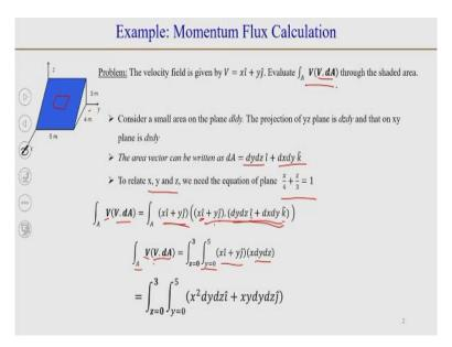
So, the first example we looked at when we were talking about mass conservation, we looked at the problem where we calculated the volumetric flow rate which is V. dA through this plane. Now, we can calculate momentum flow per unit, so if we put  $\rho$  into this then that will become a momentum flow. So, we will be calculating the integral, this integral because most of the time what we will be looking at is a, what we will be looking at is an incompressible flow.
