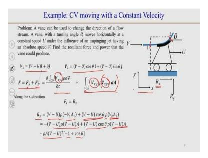
So, we have been able to find the vectors  $V_1$  and  $V_2$  which are the velocity vectors with respect to, at section 1 and section 2 these are the velocity vectors or the velocity of the jet with respect to this control volume which is moving with vane with the velocity or with the constant velocity U. Now, we can apply the momentum conservation equation to find out the velocity components or the force on the vane.
