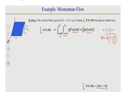
Now, when we substitute the values and because we are doing, we have the limits of y to z and we are doing integration with respect to y and z, so this x needs to be written in both the places in terms of y and z and that is where we can use the equation of plane. So, we
