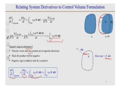
Now similarly, we do the same analysis for region 1, for region 1 the only difference that is going to come in that in this case the fluid is going to come inside the control volume, so if we consider a small region in region 1, then the flow rate here because outward normal and the velocity vectors they are in opposite direction, so the flow rate that will be coming in will be  $-\dot{V}$  dA.
