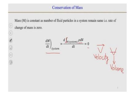
The main laws of mechanics that we will be using or that we need to use is, the first one is Conservation of Mass. So, this we might not be using very frequently to solve problems in rigid body mechanics because sometimes it is implicitly assumed that in a rigid body the mass is of course, constant, but in fluid mechanics we need to look at this. So, the first law is that in a system where the number of fluid particles is a constant, so the mass remains constant.
