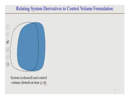
So, after time  $\Delta t$  the system moves to a different position as we can see here, the system is colored in blue and the control volume is fixed as it was at time t<sup>o</sup>. So, it remains in the same location.
