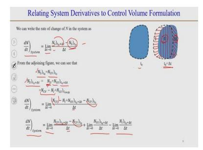
Now, we consider the motion of a particular intensive property N or what has happened to N when the system has moved from location, from the control volume from this position to this position. So, to do this we have divided the system at time  $t^{o} + \Delta t$ , in this figure we identify three regions. So, let us look at this region 1 is that is part of the control volume but the system has moved through it and we try to hatch it with kind of horizontal lines.
