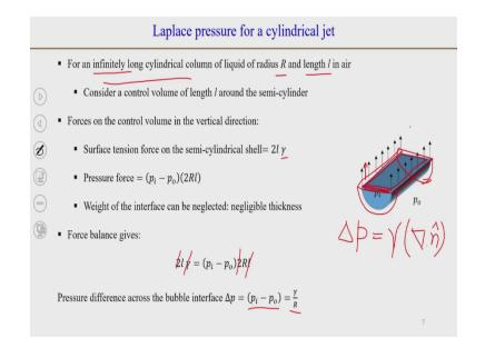
Now, if we have a cylindrical column or cylindrical jet of liquid in a gas medium, then, we can similarly find the excess pressure inside a cylindrical jet. So if we consider an infinitely long cylindrical column of liquid, which has a radius R and for the analysis purpose, we will consider a control volume of length l. So, if we consider as before for the sphere, we will consider a control volume.
