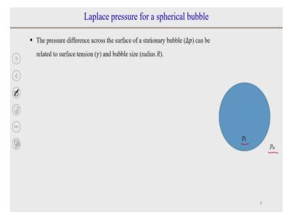
So if we take a spherical bubble of radius R and the pressure outside this bubble is po and pressure inside this bubble is pi because the pressure inside the bubble is higher than the outside pressure. So the pressure difference or excess pressure will be  $p_i - p_o$ .
