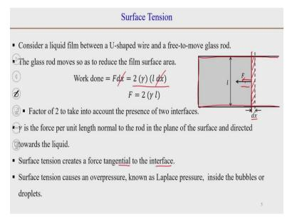
Now, this the phenomenon of surface tension or force caused by surface tension can be easily understood by an example. If we take a U-shaped wire and connect with it a movable rod, it may be a glass rod or another wire, which can move freely on this wire and dip it in a liquid or in soap water. Then, a liquid film will form. When the liquid film forms, and if we take it out from the liquid, the glass rod will start moving in this direction so as to reduce the surface area of the film.
