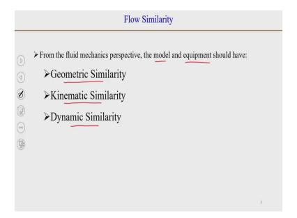
So, to achieve flow similarity, from the fluid dynamics perspective, the model and the full-scale equipment, which we will also call as prototype they should have a geometric similarity, They
