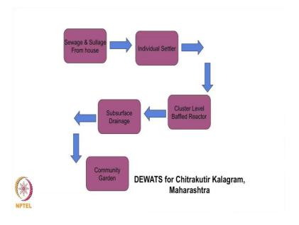
This is sewage and sullage from each house goes to an individual household levels settler and from there only the effluents are piped and they go to a cluster level baffled reactor. And after that we have just kind of let it because this was like a very spread outside, after the baffled reactor and then aerobic filter you just let it recharge the ground water because it was like about 17 acres of land and we have just 50 houses. So, this was and
