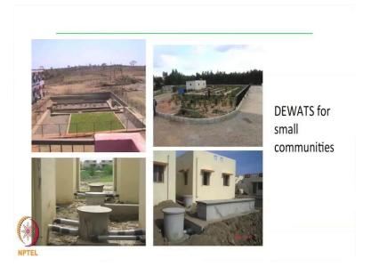
This is another small community level system, that was actually part of the Tsunami Rehabilitation Tharangambadi, where you have actually each of the houses have their own toilets. The sewage is piped and taken to a cluster level treatment system and treated actually now in Alleppey also we are doing one such similar cluster level system.
