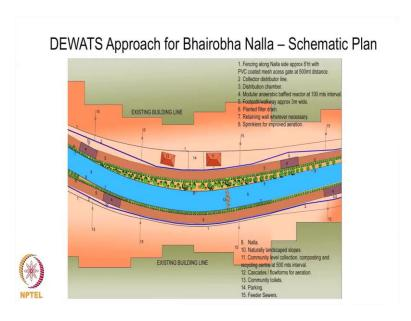
We have, so we have the anaerobic systems below the walkways on both sides and then you have the planted gravel filters along the side of the nalla. And you let the treated water into the nalla itself and you do a lot of aeration and flow forms and all that in the nalla so that, that actually helps in the further aeration of the system.
