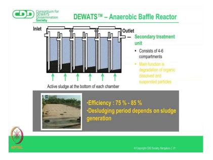
So, what we have added as a next module in the DEWATS system is something that we called as an anaerobic baffled reactor. It sounds quite complicated, but essentially it is a tank which has at least four chambers. So, what happens is that as we all know your sludge that is there in an anaerobic condition which is completely sealed and all that the sludge inside naturally develops anaerobic bacteria in about 90 days time you have started developing the anaerobic bacteria into it.
