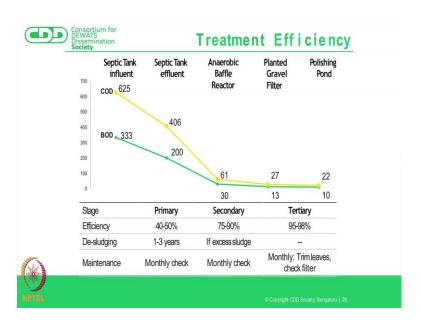
This is just a graph we just again summarizing the treatment efficiency as I said the septic tank this is the kind of if you are talking about an inlet BOD of about 330 or something, then out of the septic tank you might get this much of an efficiency. Your baffled reactor will give you this much of efficiency; the planted gravel filter you can get out BOD as I said of less than 20 and if you have a polishing pond or kind of a final
