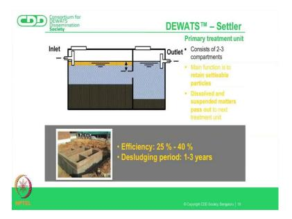
And, the connection between the first and the first and the second chamber is somewhere in the middle, so that you have the floating matter is also arrested your sludge is also separated and then you have the more of the suspended solids and bit of a sludge going into your next chamber.
