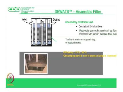
And, then the last I mean in the often in the last chambers of the baffled reactor we also add graded filter media which we call it as an anaerobic filter. So, what exactly is happening here is that the almost 75 percent treated waste water we try to give them a little more surface area for the bacteria to actually work. So, these are like again up flow chambers, but you have like a perforated slab here and you again do with an up flow so that and this is a filter media.
