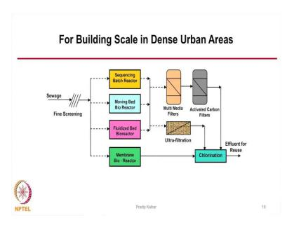
But this scheme I am explaining here at the building level, you can have the Sequencing Batch Reactor, Moving Bed Bio Reactor, Fluidized Bed Bioreactor, Membrane Bio - Reactor and which will basically take care of organic load of the sewage ok. So, first is organic load, but that will not be enough for if you want to reuse because if you are making so much of investment I said our objective should be to reuse re cycle the waste
