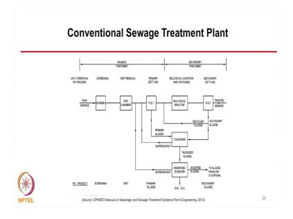
Conventional meaning it is most commonly conventionally we have to treating sewage in this manner. So, conventional treatment goes in these two primary and secondary and this particular in primary treatment we have the unit operation or process screening, grit removal and primary settling. So, in the primary treatment we take care of mostly suspended load of the particles ok. So, suspended load meaning will it remove some BOD?
