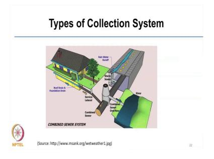
And now, this is centralized collection and treatment, where the 2 different types of collection system one is called combined sewer system where we put together the storm water. You see here storm water is connected here and mostly in Indian cities except metros city metros we have the combined sewer system because it is more economical. So, one only sewer taking the and we have very only 2 - 3 months rain fall and also some finite number of days. So, this kind of system was in India.
