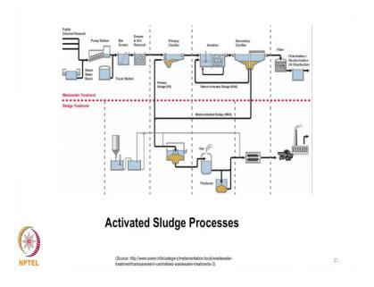
And this looks like in graphical representation this screening is happening here, bar screens are placed, then this is the grit removal ah, this is primary clarifier, you see the oxygen supply here on some external source ok. Because we have to maintain the bacteria in anaerobic mode hence we have to supply some air from the outside. And that sludge is settled and taken down for sludge processing, coming to the variants of this particular treatment systems.
