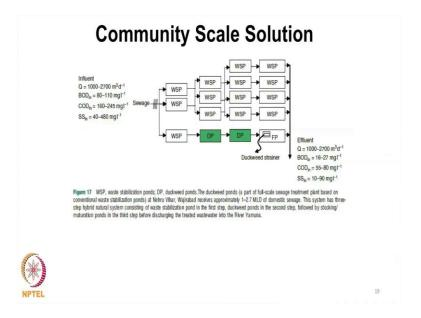
This is the waste this is the system from Nehru Vihar Wajirabad we have to check whether it is working or not, but when we documented this particular system, that was that time it was working, where you have the multiple waste stabilizations ponds. Waste stabilization ponds are natural treatment basically natural system when you have the pond there is a herbal activity and there is a symbiosis between algae and bacteria ok.
