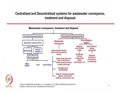
So, basically the classification for this centralized decentralized system is given in this particular book by Professor Arceivala and Professor Asolekar, where you have this centralized sewerage system which basically have the wastewater treatment plants which can be mechanized or which can be based on natural treatment system in it is centralized manner ah. And basically you can have the off site disposal or to water bodies to land or we can reuse for irrigation purposes ok.
