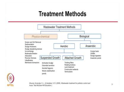
Which are like this using the physical and chemical actions or physical forces and chemical using the chemicals, which are screening, sedimentation, ion exchange, multimedia filter, adsorption, some membranes reverse osmosis and this all have has it is own particular unique purpose and when to use and when not to use.
