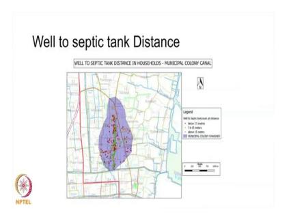
And this is the when to septic tank distance which we have measured earlier, now when we couple it with the water quality analysis. We can see that out of the dug wells out of the whole number of dug wells around 261 of them were tested for water quality and almost 93 percent of them had E coli contamination which is a same in most parts of Kerala. If you look at ground water, it is contaminated and it make sense there was no
