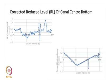
As I told you this is the canal profile of the Marthoma Church sub canal, you can see there are a lot of undulations here and this is the corrected level of the corrected reduced level of the sub canal.
