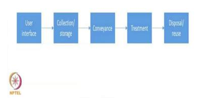
So, now, coming to the sanitation service chain; are you are you familiar with this picture? So, this is the sanitation service chain which is happening, this is the standard sanitation service chain where the first there is a user interface. There is the collection and storage system, conveyance, treatment and disposal and reuse, this is this applicable to Alleppey? You think so?
