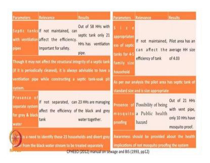
So, we are asking a question on whether the septic tanks with ventilation pipe or not. So, if not maintained if a set a ventilation pipe is not maintained, it can affect the efficiency of the septic tank and also it can provide the to be a problem to the structural integrity of the septic tank ok. Ventilation pipes they release all the byproducts anaerobic reaction, H2S and methane into the air and not having it might affect the integrity.
