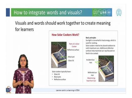
Here is another example of how visuals and words can work together to create meaning for the learners. We can see that the concept of solar cooker has been effectively captured in this image. The image not only shows a different parts of solar cooker, it also shows how the sunrays are captured the incident and the reflected rise are captured to help in the cooking.
