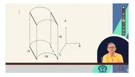
So, that is at r. That is why it is coming that out at r plus delta r is equal to  $m_r$  into A plus del del r of  $m_r$  into del r into the area r plus del in del theta del z, right. r plus del r is the other arc, right. This arc is r del theta, and that arc is r plus del r del theta del z, ok. So, now this is equal to  $m_r$  into r plus del r into del theta del z plus del  $m_r$  del r
