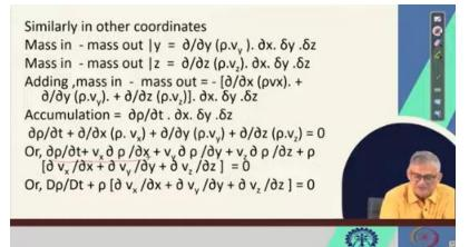
Now, this D rho D t plus rho del  $v_x$  del x plus del  $v_y$  del y plus del  $v_z$  del z, this becomes equals to 0, right. So, the substantial time derivative we can write, capital D rho capital D t plus rho del  $v_x$  del x plus del  $v_y$  del y plus del  $v_z$  del z equals to 0, right. Now, if the fluid is incompressible, then D rho D t is constant, which we have also seen earlier, that is
