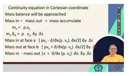
So, m dot x into delta A or  $m_x$  into delta A is rho  $v_x$  into the area of the x face. The x face area is  $\Delta y$ ,  $\Delta z$ , right. That we can check by looking at the screenshot 1. This was, right, in the x. So, it is in the x, this is the face, ok. So, this face is del y del z. Similarly, this at x plus  $\Delta x$ , this face area is  $\Delta y$ ,  $\Delta z$ , right.
